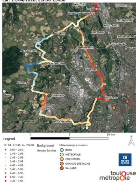
Urban Heat Island measurement with instrumented car. 17/04/2018, 21h30-23h30
