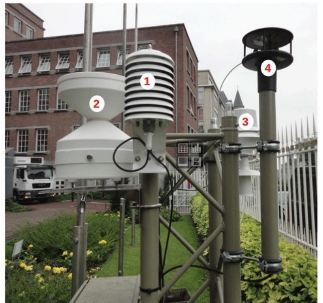
Detailed view on the sensors of one of the weather stations: actively ventilated radiation shield (1) with temperature sensor, rain gauge (2), passively ventilated shield (3) with temperature, and relative humidity measurement and ultrasonic anemometer.
